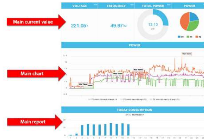
Report workshop energy consumption
